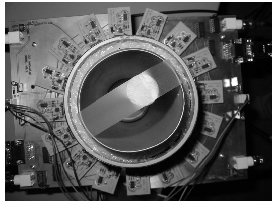
Figure 4: Dielectric cylindrical rod placed near the center of the tube. The electronics for the 16 electrodes can be seen as well.
